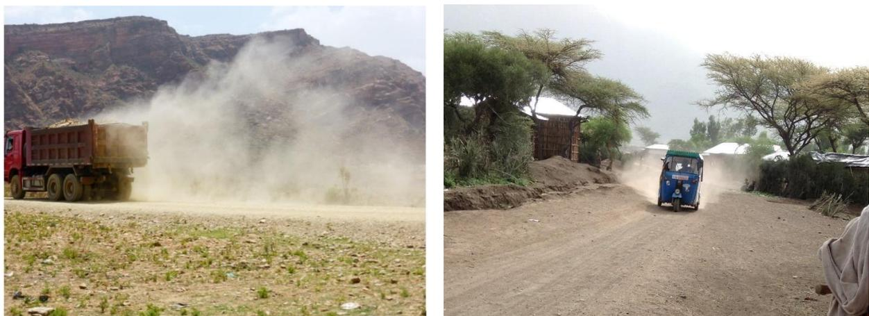
Figure 14: Dust lifted up by heavy truck and even by bajaj in Tigray region
